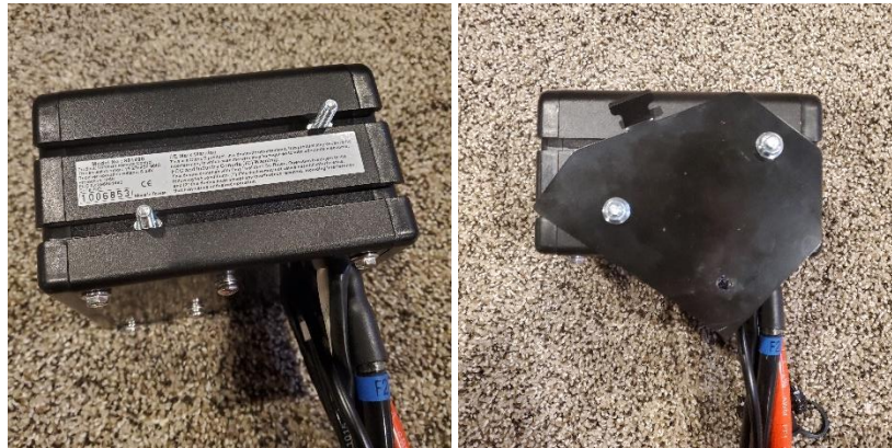
Bolt locations in controller t-slot for backplate
