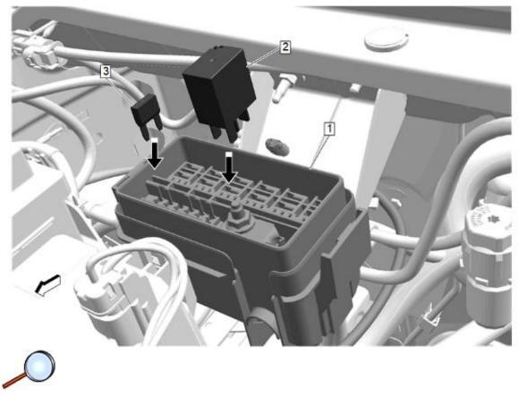
14. Locate relay (2) and fuse (3) from kit and insert into appropriate area defined by instruction accessory VBP fuse box (1). Refer to <u>Accessory Wiring Junction Block Package Installation</u>.
