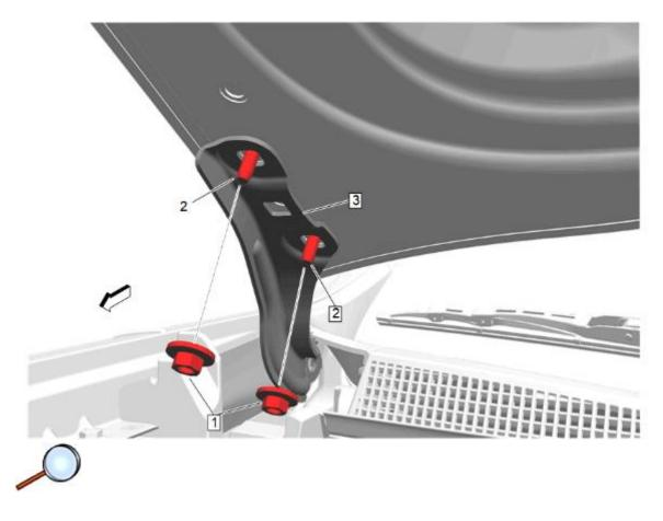
Note: Do not remove hood hinge nuts on opposite side at this time.
