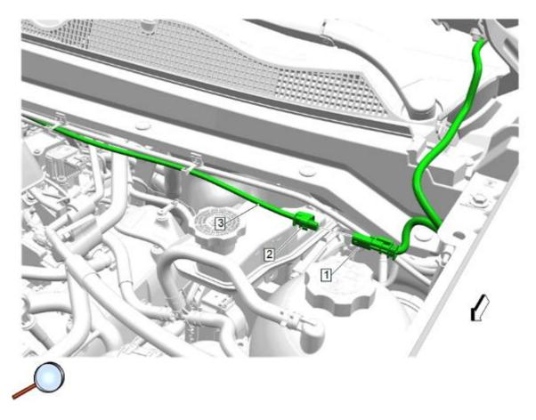
10. Continue to route harness (3) to driver side of vehicle and connect driver side lamp electrical connector to harness electrical connector (2).
