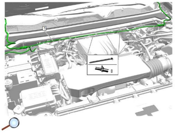
11. Secure harness (1) to existing harness under the air inlet panel using supplied tie straps every 200mm.
