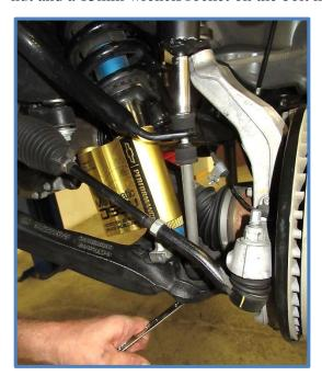
3. Remove the nut from the upper control arm ball joint using an 18mm socket and separate the upper control arm from the knuckle/spindle.
