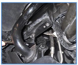
14. Bolt the sway bar to the sway bar plate using the supplied 3/8" x 3/4" bolts and tighten with a 9/16 socket.
