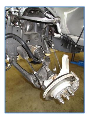
7. Installing King Shocks – Be aware the shocks are side specific, make sure you are installing the proper shock on the correct side (see pics below for reference). Place the shock in position on the vehicle and install the provided 10mm lower mounting bolts w/washers. Insert bolts up through the lower mount, install the washers and nuts and tighten to 40 ftlbs.
