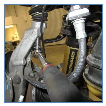
4. Remove the two lower mounting bolts using a 15mm socket.
