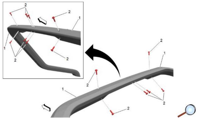
10. Attach the tube connector to both rear tubes (1) using fourteen M6 torx fasteners (2). Tighten the fasteners to  $10 \pm 1$  N.m (7 lb ft).
