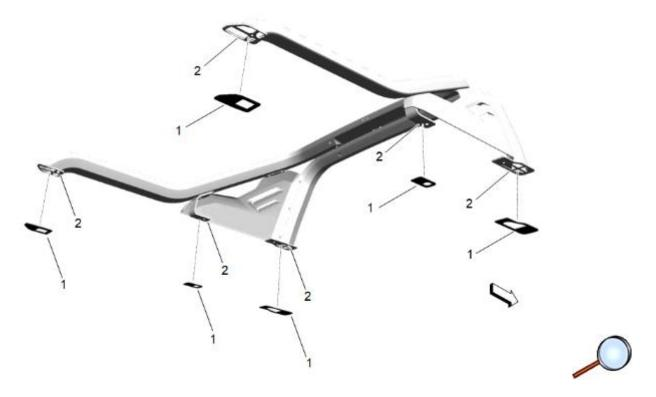
16. Peel off the white adhesive backer and position the foam gaskets (1) to the matching areas on the sport bar assembly (2).
