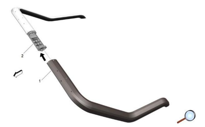
9. Insert the tube connector (2) into the LH rear tube (1).
