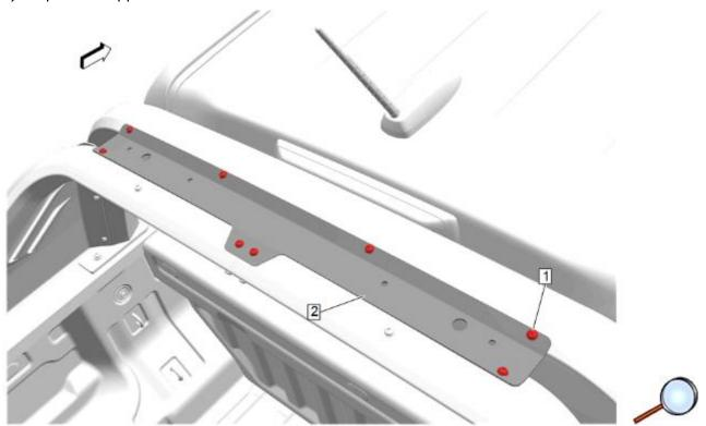
25. Tighten the eight M6 torx screws (1) that secure the top plate to the front and rear tubes to  $10 \pm 1$  N.m (7 lb ft).
