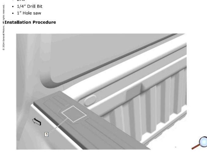
1. Carefully cut the bed rail molding (1) along the rectangular grooves to expose front stake pockets.
