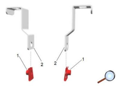
18. Attach J-nuts (1) to the rear stake pocket brackets (2).
