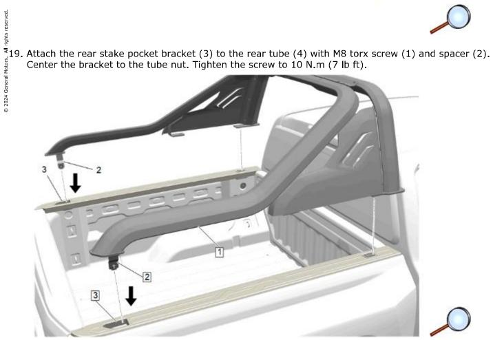
20. With the aid of an assistant, position the rear stake pocket brackets (2) into the rear stake pockets (3) and position the sport bar assembly (1) to the vehicle.
