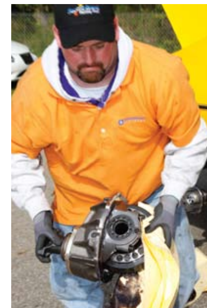
> When the ZZ4 small-block was swapped in, the 4.44:1 rear gear used for the LS7 and LS3 engines was exchanged for a 4.30:1.
