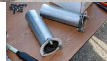
> On the LS and small-block engines, these 9-inch exhaust collector extensions were usually good for around a half a tenth. A little longer (like 12 inches) would probably be even better, but the crossmember was in the way and there was insufficient time to develop a workaround.
