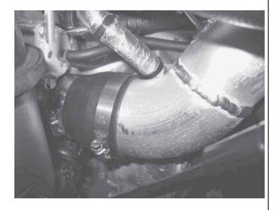
2u. Using a zip tie, gently take up the slack between the factory MAF harness wire and the rubber hose.
