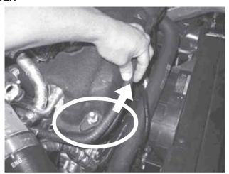
2i. Install Induction Tube, place the MAF sensor side of the tube into the front portion of the engine bay as shown.
