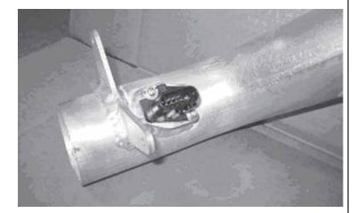
2g. Install the 2 push mount zip ties, one in each hole of the two small tabs on the induction tube as shown below and secure MAF harness extension, but do not fully tighten zip ties yet. Plug the extension into the MAF sensor.
