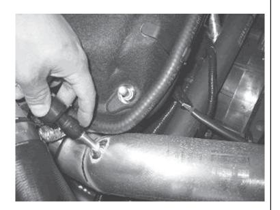
2s. Position size 48 clamp on the reducer coupler as shown and tighten
