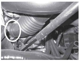
1c. On the passenger side of the vehicle. Remove the bolt and two nuts circled. Remove both brackets. (apply lubricant to the rubber grommet when removing). Repeat this step for the driver side.
