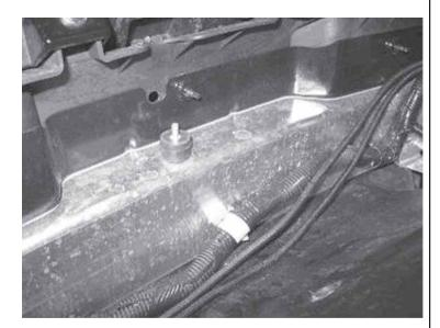
2c. Install front mount bracket and loosely install a 6mm serrated nut, do not fully tighten the nut yet.
