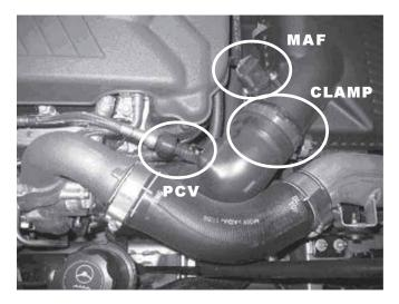
1b. Loosen both clamps holding the factory induction tube.
