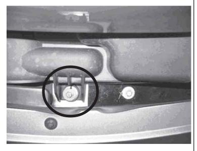
1g. Remove lower portion of the air box. Both aluminum turbo intercooler tubes can tilt outwards (see arrows) allowing clearance needed for removal. When the air box is removed, re-install factory hardware removed in step 1c and 1d.
