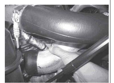
21. Install the Air Filter Pre Filter onto the filter and install both onto the induction tube and secure with a size 52 clamp.
