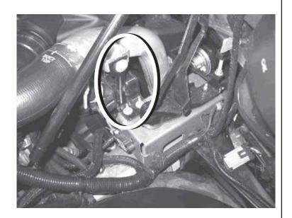
1d. Remove both bolts circled in photo. This will allow the turbo intercooler tubes to tilt outward enabling the lower section of the factory air box to be removed.
