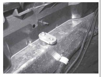
2d. Insert M6 bolt from the bottom up, place a 6mm washer on top of the bracket and lightly secure using a 6mm serrated nut, do not tighten yet.
