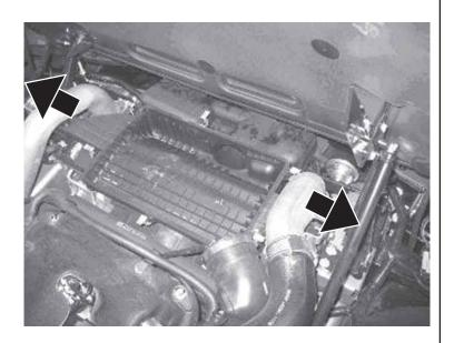
1f. Undo the 6 circled metal clips and remove the top portion of the air box and remove the panel air filter. Also, remove the factory induction tube leading to the turbocharger inlet and the engine cover by pulling upwards at the 4 corners of the cover.
