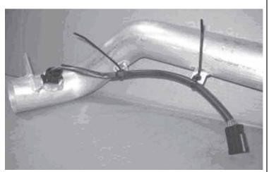
2f. Install MAF sensor onto the GM Performance Induction Tube | 2h. For additional clearance, reposition the rubber hose pictured so the bend on the hose is closer to the valve cover.
